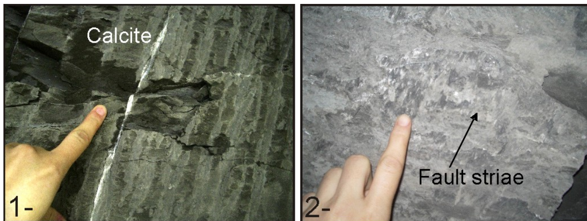
Figure 4. Tectonic structures observed on Tournemire drift walls: 1- calcite vein, 2- normal fault striae
